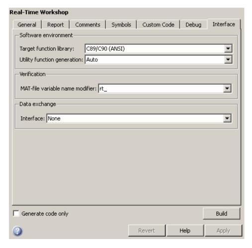
The Real-Time Workshop Interface pane includes the following parameters when the Real-Time Workshop product is installed on your system and you select an ERT-based target. ERT-based target parameters require a Real-Time Workshop Embedded Coder license when generating code.
