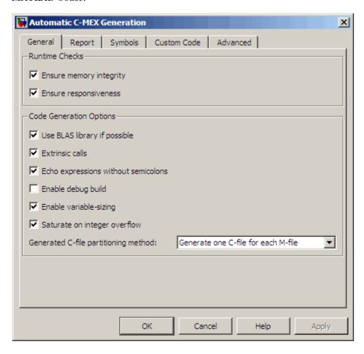
The following table describes the general parameters for the Embedded MATLAB Coder Automatic C MEX Generation dialog box:
